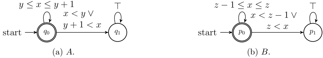
Figure A.1: Two PA that are deterministic per assignment and describe the language L_3 .
