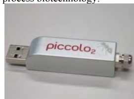
Optoelectronic system containing an RSB port (left) and a fiber connector (right) for fiber optic decay time-based sensing of O 2 .
