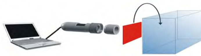
Schematic of the state of the art in imaging O 2 . Left: PC with software and for display. Center: Handheld portable instrument for lifetime imaging. Red film: Sensor membrane incorporating a quenchable luminescent probe for O 2 to be placed on the object of interest (a bioreactor, or skin, or an aircraft, etc.; symbolized by a cube)
